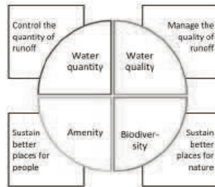
Figure 1. According to CIRIA [11] multifunctionality of sustainable urban drainage systems (SUDS) based on the simultaneous existence of four criteria; quality and quantity control, biodiversity, and amenity. However, any mutual interconnections are not presented (figure adapted from CIRIA [11]).
