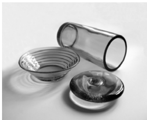
Figure 2. Products made from EOL colour panel glass with different production techniques (blown cylinder, centrifugal casted bowl and casted candleholder).
