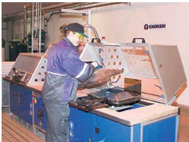
Photo 4. Dismantling of the funnel and panel parts by hot-wire technique. Photo: Ekokem Oy Ab
