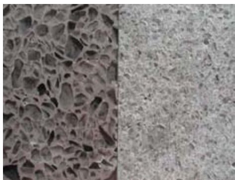
Figure 3. Construction blocks of 95% colour panel glasses. The variation in the colour hue has been achieved with different particle size distribution of the glass material.
