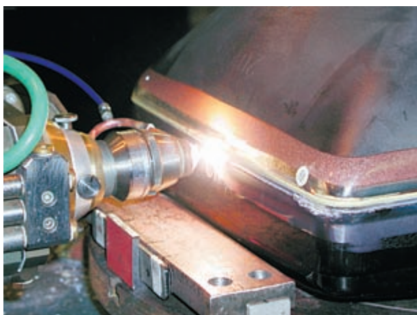
Photo 5. Dismantling of funnel and panel parts by laser cutting technique in the Proventia Automation Oy's plant. Photo: Proventia Automation Oy
