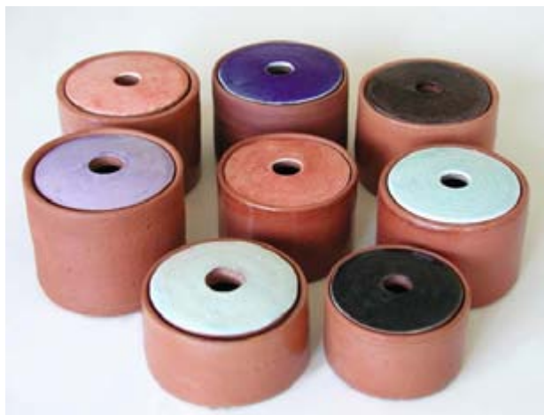
Figure 2. Products made by throwing out of Finnish earthenware and glazed with clear and coloured test glazes. Glazes contain 95 weight-% of EOL CRT glass.
