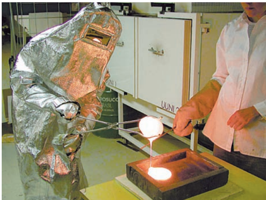
Photo 6. Test melting of Cathode Ray Tube glass at University of Art and Design Helsinki Photo: Satu Typpö.
