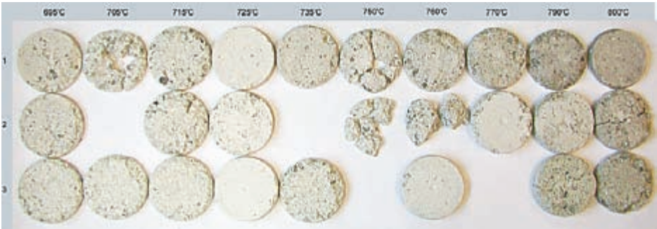
Photo 10. Photo of gradient-fired test samples for glass tiles. Test samples with three different batches containing various particle size fractions were fired in the temperature range 695–800°C. Photo: Kirsti Taiviola.
