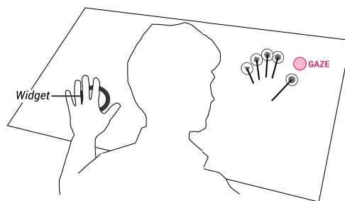
Figure 1. We use the combination of above-surface sensing and eye tracking to facilitate direct input, even when the user is not visually attending to the target. The system determines potential user actions through above-surface sensing, but defers their confirmation to touch input, accompanied by gaze-adaptive visual feedback between these two steps.
