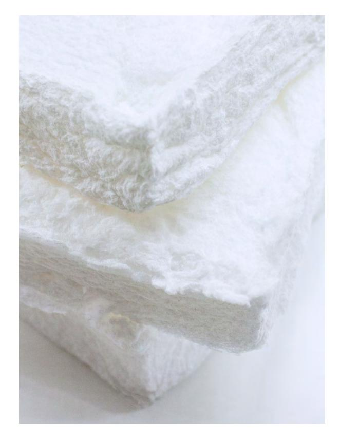
Foam forming is a new technology that enables the effective production of a vast range of fibre-based materials. The bubble structure of wet foam gives a handle to control the spatial distribution and orientation of fibres inside the foam. By feeding the fibre foam onto a porous fabric and then sucking out the wet foam, one is left with a fibre network that forms the skeleton for a lightweight material.
