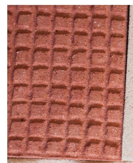
When wood-dust is mixed with nanocellulose, the new material can be called 'Casted Wood'. In the future similar material could be used in 3D printing. Various samples have been produced by Heidi Turunen.
