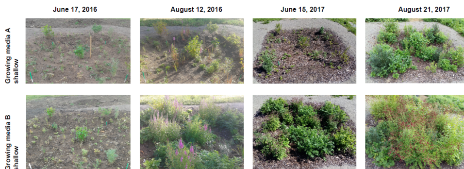
Figure 10. The development of vegetation cover in shallow cells with growing media A and B. The first photos were photographed one week after planting. Growing medium A showed light growth (upper row) when compared to the media containing compost and topsoil (lower row).
