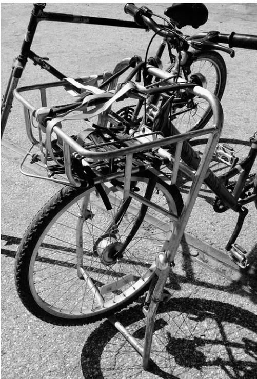
Figure 7: Metal scraps were collected and welded as a protective cover against strong impacts.
