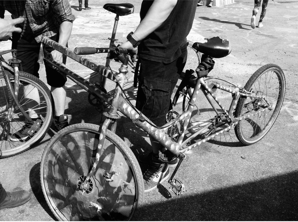
Figure 8: After welding two frames and several metal sticks together, they were looking for suitable rims.
