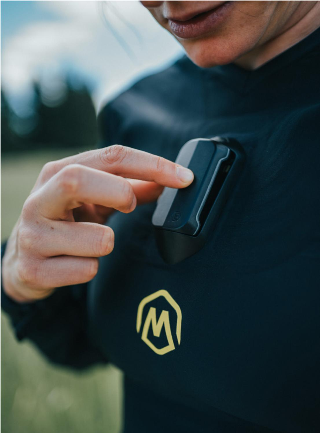
FIG. 34 · Myontec's smart sportswear measures muscle activity by using silver-coated fabric and sewn-in sensors. The garments are used in elite sports coaching to analyse performance and muscle recovery during sports or, for instance, after injury. Photo: The Czech Ergonomics Association.
