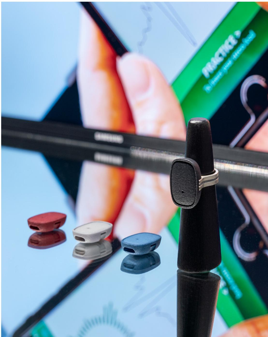
FIG. 36 · The Moodmetric ring and the related app measure and interpret the electrodermal activity (EDA) signal that reflects the activation of the sympathetic nervous system (SNS). SNS activation directly influences sweat gland activity and this change can be measured as variations in skin conductance. The measurement is done with the help of two electrodes placed on the skin through the ring.
