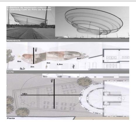
Figure 7: Section and plan of design project proposal for the outer space of E-Learning Café of Asprela
