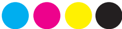
The four process colours (CMYK) traditionally used in printing cyan, magenta, yellow, black
