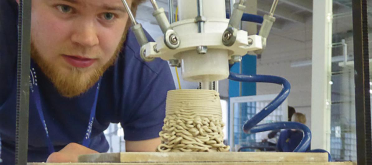
left: Fig. 2 A long distance between the coiled layers or high pressure on the clay extruder results in a softly curved layering with an ornamental effect.
