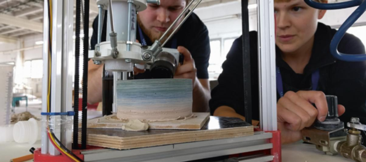
Fig. 1 Controlling the pressure while printing makes it possible to change the size and expression of the coiling.
